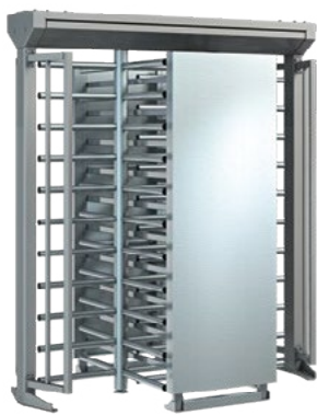
Kentaur FTS-L01 Double turnstile separation segments: 90°, with stainless steel straight crossbars, steel middle section and stainless steel-clad front sides, satin matt finish, low space requirements thanks to interlocking rotating units
