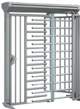
Kentaur FTS-M03 Turnstile separation segments: 180°, with stainless steel straight crossbars, polished. Integrated full-height gate for on-request opening with straight crossbars and continuous frame. With steel columns and climb-over protection
