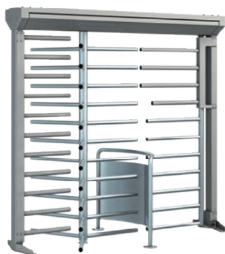
Kentaur FTS-M01 Turnstile separation segments: 120°, with stainless steel straight crossbars, polished. Waist-high, made of curved tubular stainless steel with plate panels, automatic bicycle gate
