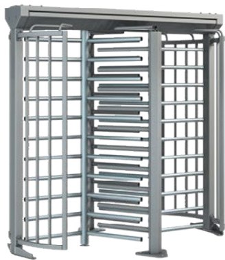
Kentaur FTS-E06 Double turnstile separation segments: 120°, each with stainless steel straight crossbars, polished. Low space requirements thanks to interlocking rotating units
